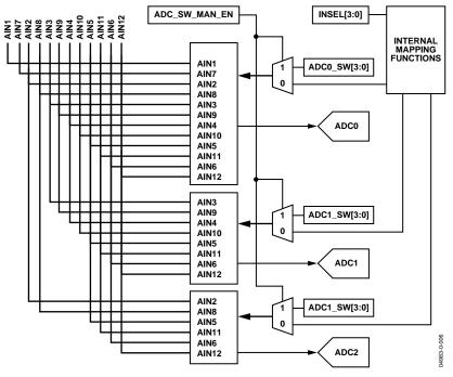
Figure 6. Internal Pin Connections
