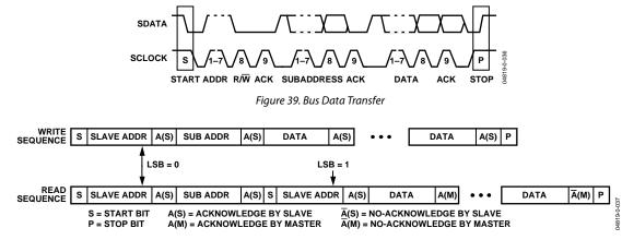
Figure 40. Read and Write Sequence
