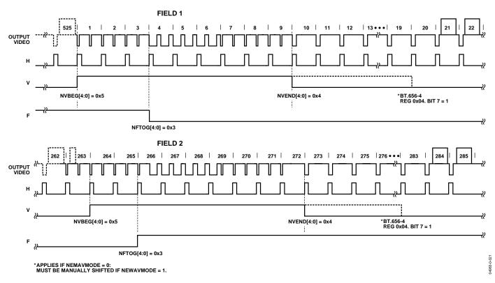
Figure 21. NTSC Default (BT.656). The polarity of H, V, and F is embedded in the data.
