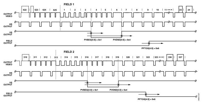
Figure 27. PAL Typical VSync/Field Positions Using Register Writes in Table 56
