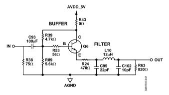
Figure 44. ADI Recommended Antialiasing Circuit for All Input Channels
