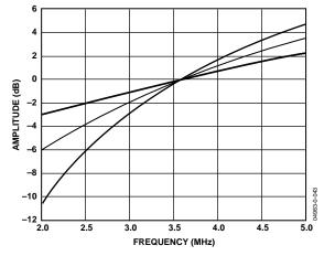
Figure 36. NTSC IF Compensation Filter Responses
