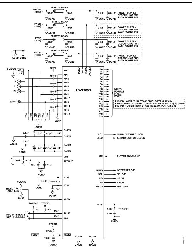
Figure 45. Typical Connection Diagram
