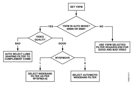
Figure 11. YSFM and WYSFM Control Flowchart
