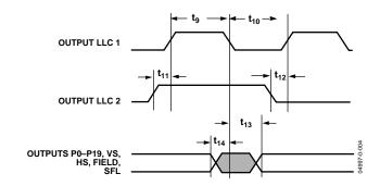
Figure 3. Pixel Port and Control Output Timing
