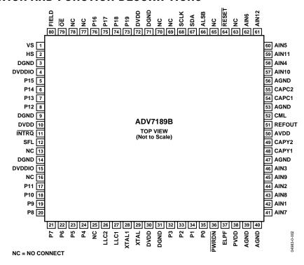
Figure 5. 80-Lead LQFP Pin Configuration
